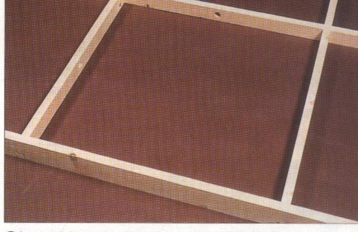
Lay out the parts on a flat surface and it's easy to see how they fit together, all the cut-outs interlocking. At this point the joints can be opened, PVA wood glue applied and fitted back together again before being fixed with the pins supplied.
